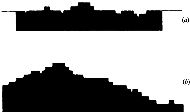
Fig. 1.9. Surface morphology: (a) T < T_r ; (b) T > T_r (Muller-Krumbhaar, 1978).
