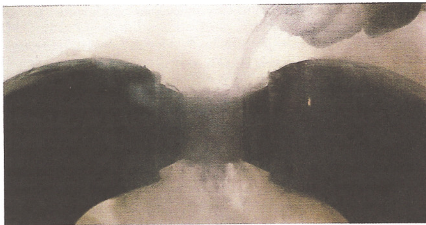
Figure 13-6 Liquid oxygen is attracted to the magnetic field between the poles of a magnet because oxygen is paramagnetic.
